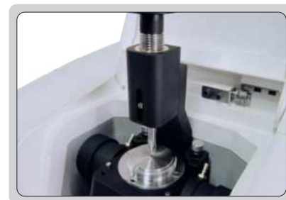
ZnSe crystals ATR attachment (included)
