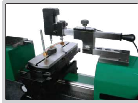
thread ring gauge measurement
