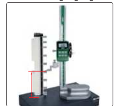
check height gauges
