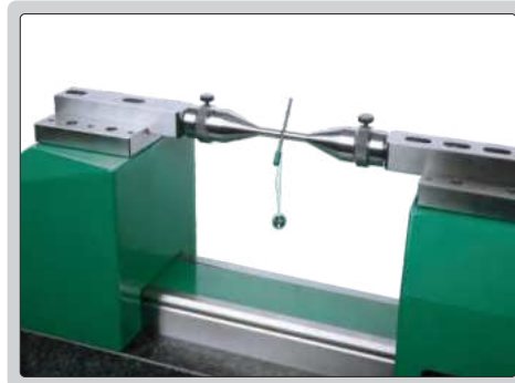
pin gauge measurement
