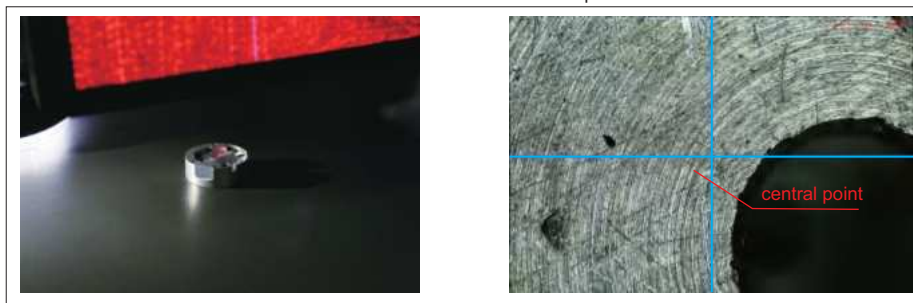
laser indicator locates the central point
