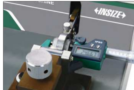
lapping measuring surfaces of outside micrometer
