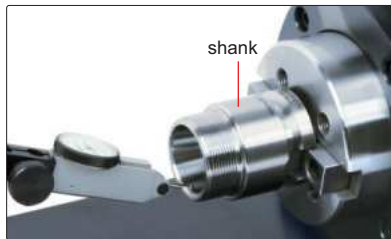
measure radial runout of shank
