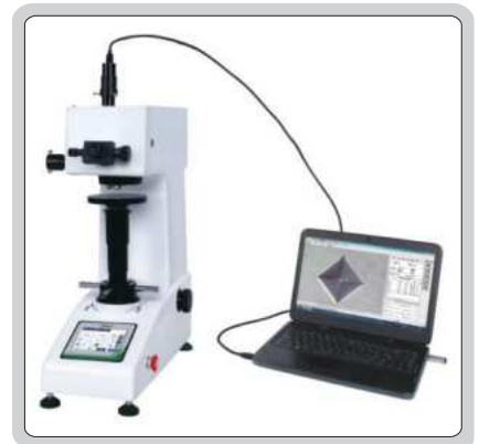
camera and measuring software (optional)
