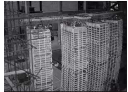
deformation monitoring of large building vibration test
