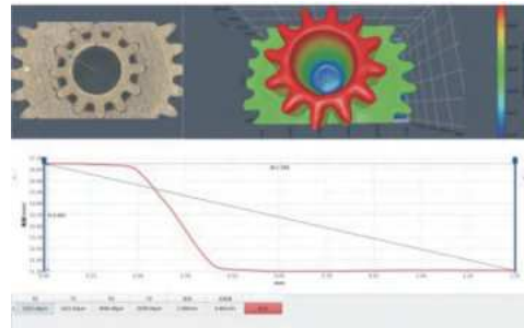
measurement of component bore height
