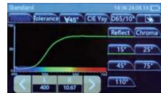
specimen reflectance recording interface
