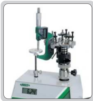
check the measuring force of micrometers
