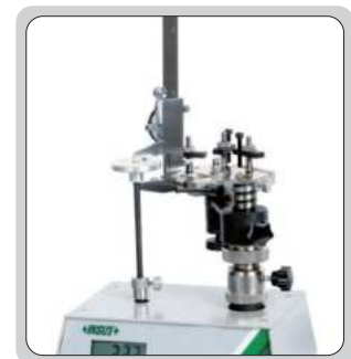
check the measuring force of calipers
