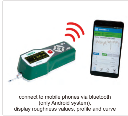
operate roughness tester by mobile phones
