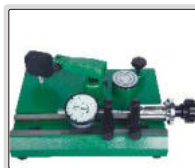
inspect accuracy of dial indicators (range 0-25mm)
