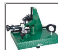
test the effect of lateral force on accuracy of test indicators (half round gage block is required)
